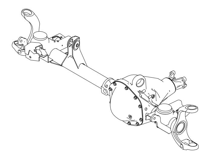
Step 3: Trim driver side upper control arm mount so that you have 2 posts that fit into the 2 cut outs in the top of the bridge about an 1/8" below the top of the bridge. Step 4: Bevel the bridge where the axle tube goes so it clears the welds on the spring perch.
